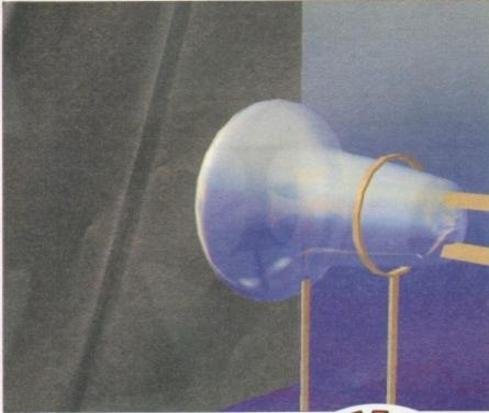
This early design of cathode ray tube shows a Maltese cross working as the anode, projecting its image onto the screen
